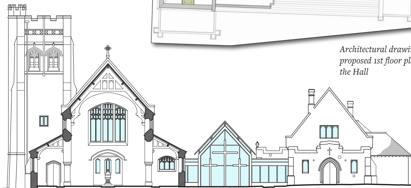
Architectural drawing showing how the new development will link the Church and hall
